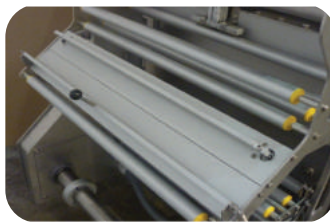
Built in Film Splice Included in Unwind Frame
