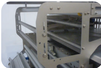
Unwind Frame designed to accept Printer
